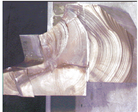
Fig. 2-1. Shaft crack caused by an out-of-step condition.
